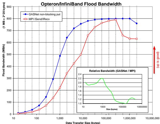
Figure 3. Bandwidth of GASNet vs. MPI on InfiniBand
