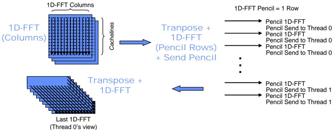
Figure 6. 3D-FFT by communicating overlapping pencils
