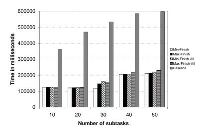
Figure 9. Simulation results for 20 machines and 6 data repositories with varying number of subtasks
