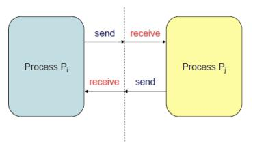
$\begin{array}{l} \text{naming} \\ \text{(direct)} \end{array} \begin{cases} \text{send(P}_j, \text{ message): P}_j \text{ identifies process j in the system} \\ \text{receive(P}_j, \text{ message): P}_i \text{ identifies process i in the system} \\ \end{array}$
