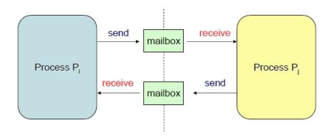
$\begin{array}{l} \text{naming} \\ \text{(indirect)} \end{array} \begin{cases} \text{send(m_a, message): m_a identifies mailbox a in the system} \\ \text{receive(m_b, message): m_b identifies mailbox b in the system} \\ \end{array}$
