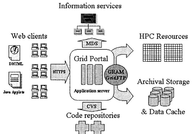
Figure 2. Grid Portals provide a central point of access to widely distributed Grid services.
