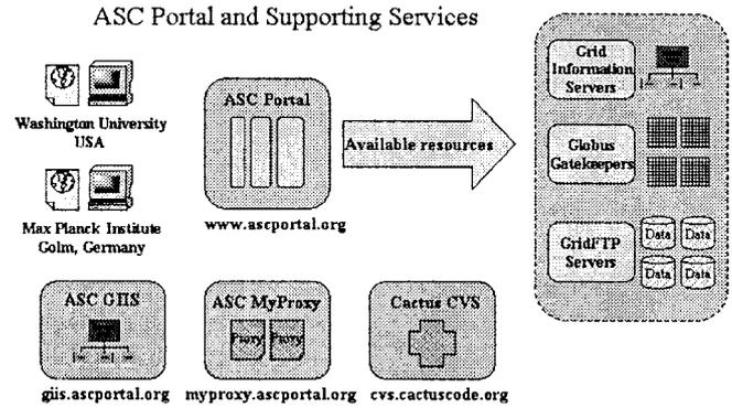
Figure 5. The ASC Portal is supported by a variety of Grid services and technologies.
