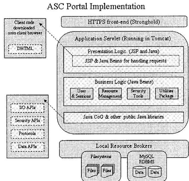
Figure 6. The ASC Portal server-side architecture and its software components.
