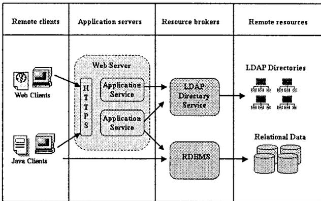
Figure 4. N-tier applications divide functionality into layers in order to maximize the sharing of resources and services among clients.
