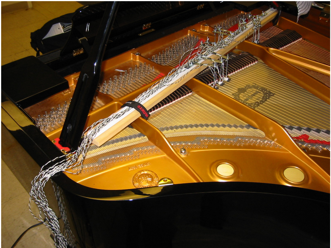
Figure E.8: Electromagnetically prepared piano prototype
