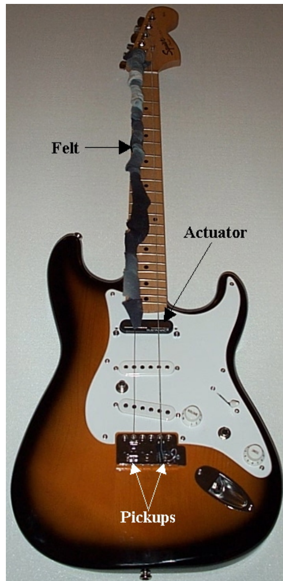
Figure E.5: Tangible Guitar String Interface
