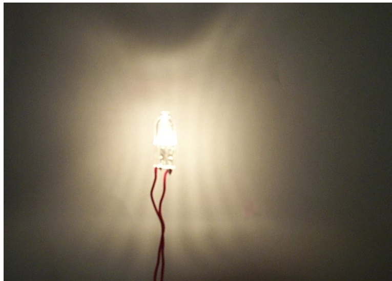
Figure F.11: Nonuniform radiation pattern of a coiled halogen lamp
