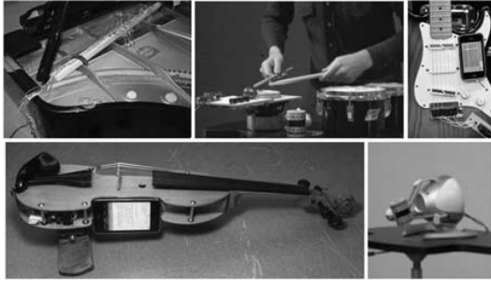
Figure 1. Clockwise from top left: the Electromagnetically Prepared Piano, the Haptic Drum, the Feedback Resonance Guitar, a teleoperated acoustic shaker held by the Falcon force-feedback device, and the Overtone Fiddle.
