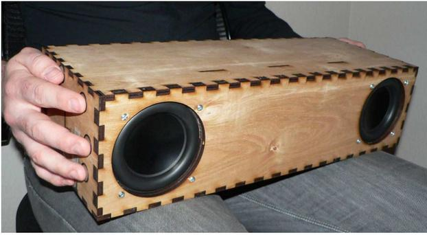
Figure 5: *LapBox* revision 3, with force-sensing resistors placed on the sides in the shape of the human hand.
