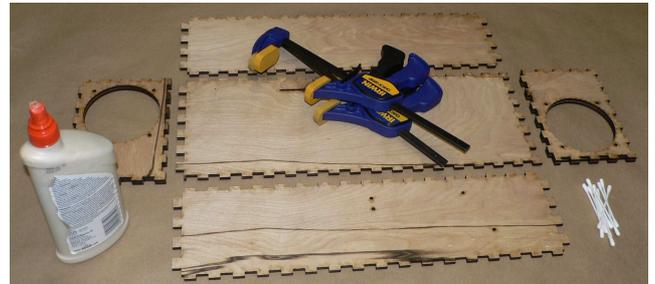
Figure 2: Preparations for gluing together pieces of laser-cut plywood to make an enclosure.
