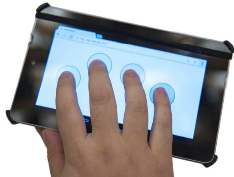
Figure 5: Multi-touch interaction with a Nexus tablet controlling sound synthesis on Satellite CCRMA via Interface.js .
