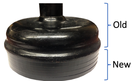
Figure 4. For Hang-ups , the old telephone base needed to be extended with some new acrylic discs in order to house the additional electronics.
