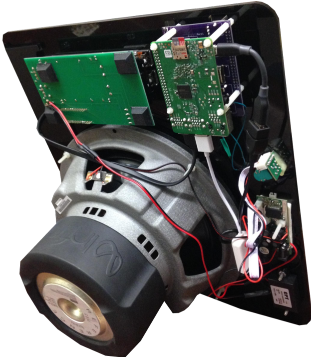
Figure 5. This example dipole instrument can stand up on a table exposing the electronics, which makes it easy to work on it.
