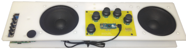
Figure 8. A dipole instrument for playing a pair of coupled circle maps [23, 24] as connected to a pair of digital waveguides [22].
