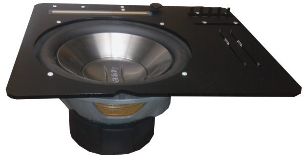
Figure 3. An example dipole instrument (loudspeaker has diameter, 12" (30.5cm)) that can balance upright by itself on a table (electronics hidden underneath the black acrylic plate).
