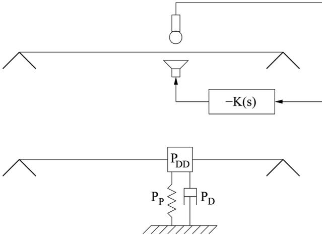
FIG. 5. Control of a vibrating string with a collocated sensor (depicted as microphone) and actuator (depicted as loudspeaker) (top); Mechanical analog of PID control (bottom).
