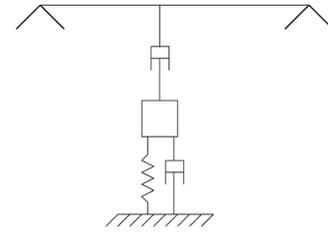
FIG. 9. Mechanical physical analog of the notch controller.
