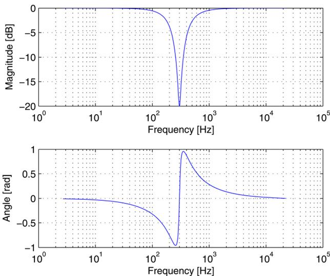
FIG. 8. (Color online) Frequency response of the notch filter controller given by Eq. (10) with  $f_c = 300$  Hz,  $\tilde{Q} = 1$ , and  $\alpha = 10$ .
