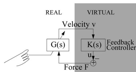
FIG. 3. Feedback loop shown from controller's perspective, with the controller represented by the Laplace-domain transfer function  $K(s)$ .
