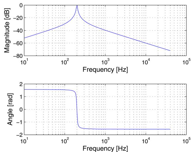
FIG. 6. (Color online) Frequency response of the bandpass controller given by Eq. (9) with  $Q = 20$  and  $f_c = 200$  Hz.
