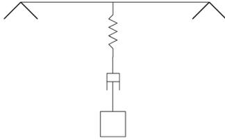
FIG. 7. Mechanical analog of the bandpass controller.
