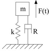
FIG. 4. Model for musical instrument resonance with equivalent mass  $m$ , damping parameter  $R$ , spring constant  $k$ , and external force  $F(t)$ .
