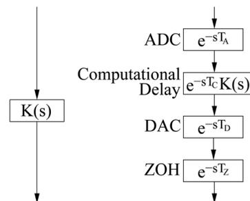
FIG. 10. Ideal representation of controller (left); digital approximate implementation of controller (right).
