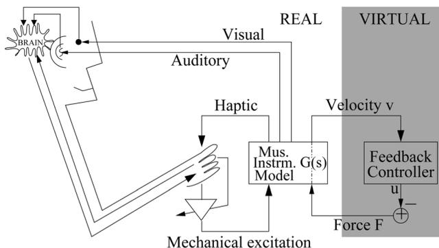
FIG. 2. Musician interacting with a feedback controlled acoustic musical instrument.
