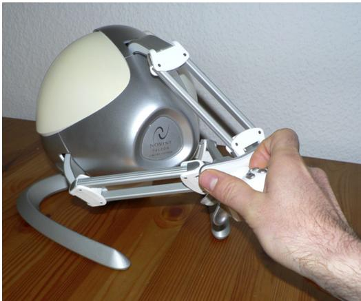
**Figure 1.** NovInt Falcon haptic force-feedback device.
