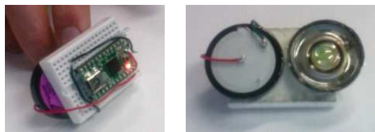
Figure 3: Teensy on breadboard (left) with 3.3V battery and loudspeaker on underside (right)
