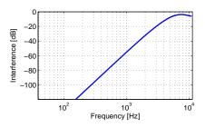
▶ The estimator is accurate and the interference from the left-going traveling wave is more than 50dB down for  $f \in [0kHz \ 1.2kHz]$ .
