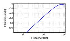
► Consider c = 400m/s and M = 5 sensors with spacings -8cm, 4cm, 0cm, 4cm, and 8cm.
