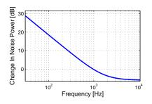
► The sensor noise power increases by more than 12dB below 200Hz.
