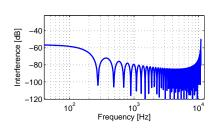
The estimator has 0.8dB of ripple for  $f \in [0.2kHz \ 10.2kHz]$
