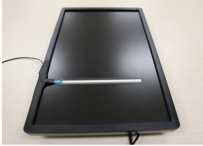
Fig. 2. The experimental apparatus provides a display with colocated sensor for target performance.
