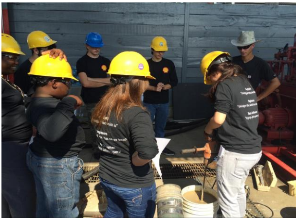
Teams preparing the mud for the U-Tube and measuring its density. PERTT LSU
