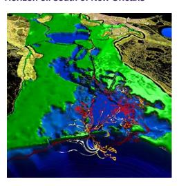
Caption: A map of the Barataria Bay estuary depicting the simulated movement of surface oil slicks in the aftermath of the Deepwater Horizon oil spill. Visualization by Dr. Werner Benger (LSU Center for Computation & Technology). Model bathymetry and oil spill simulations by Dr. Dubravko Justic and Lixia Wang (LSU Department of Oceanography & Coastal Sciences).
