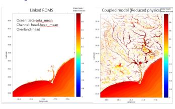
In coupled modeling, simulations of river and ocean are paired and run at the same time, so each receives feedback from the other. This recreates the conditions of a compound flooding event, where the storm surge accompanying the landfall of a hurricane and the swell of rain-induced flooding as the storm moves inland meet over a coastal area.
