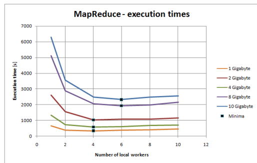
Fig. 4: Plots showing how the T_c for different data-set sizes varies with the number of workers employed. For example, with larger data-set sizes although t_{pp} increases, as the number of workers increases the workload per worker decreases, thus leading to an overall reduction in T_c . The advantages of a greater number of workers is manifest for larger data-sets.
