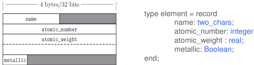
Figure 7.1: Likely layout in memory for objects of type element on a 32-bit machine. Alignment restrictions lead to the shaded “holes.”
