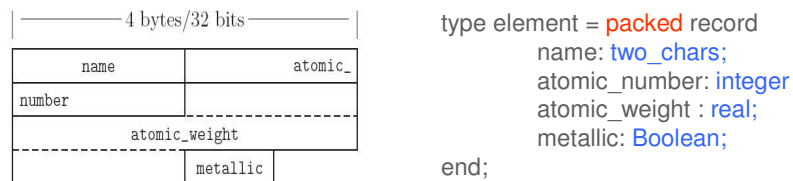
Figure 7.2: Likely memory layout for packed element records. The atomic_number and atomic_weight fields are nonaligned, and can only be read or written (on most machines) via multi-instruction sequences.
