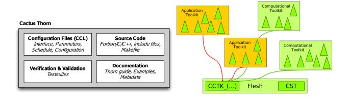
Figure 1: [Left] Internal structure of a typical Cactus component (thorn). [Right] High level view of a typical Cactus application, where the Cactus Specification Tool (CST) provides bindings between thorns and the flesh. The Cactus Computational Toolkit (CCTK) provides a range of computational capabilities, such as parallel I/O, data distribution, or checkpointing via the Cactus flesh API.
