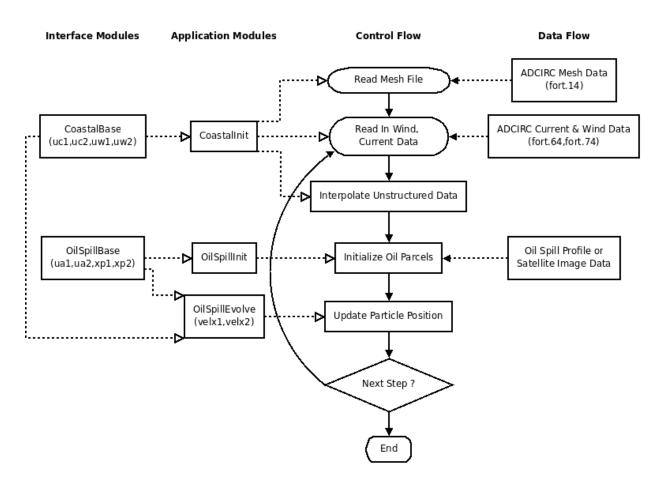
Figure 2: The oil spill modules can be separated into two groups. The interface modules define fundamental variables that can be shared among different modules. The application modules define operations that can be applied to the fundamental variables. Each application module is in charge of one or more tasks in the overall work flow and is responsible for its own input data.
