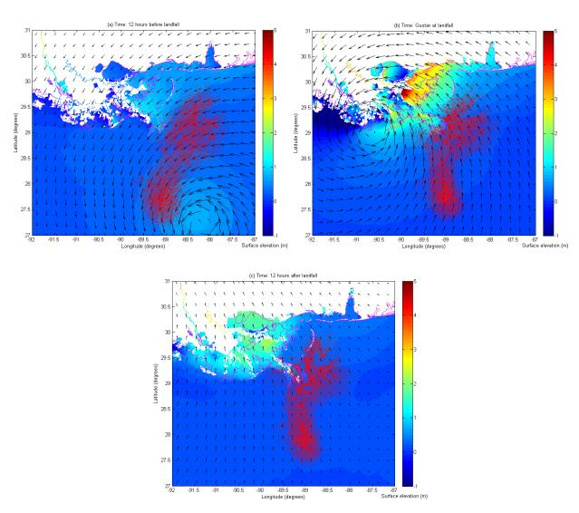
Figure 5: Visualization of a gulf coast oil spill simulation with Gustav hurricane data at three different time steps (down-sampled by a factor of 50). The red points represent oil parcels, and the black arrows represent horizontal wind velocity field 10 meters above the ocean surface. The length of the arrows is proportional to the wind speed. The background is the storm surge distribution. The interval of contour line is 0.1m.
